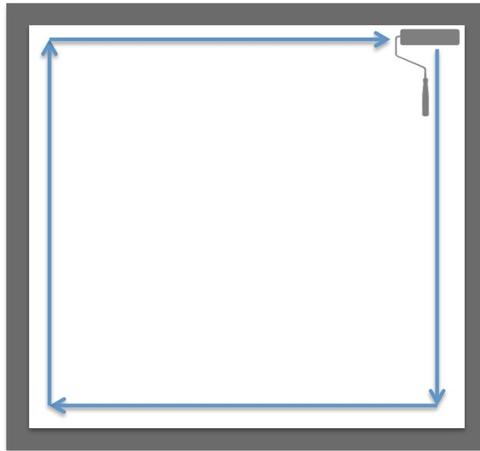
The next passes will be a vertical motion from the top to the bottom of the area, then from the bottom to the top of the area repeatedly in a “V” pattern while slightly overlapping each roll. Avoid sliding the roller.
